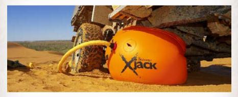
The Bushranger X-Jack was also a standout, it took home the Best New Exterior Accessory award. The X-Jack is ideal for vehicle recovery in sand, mud or snow, and is operated by connecting the X-Jack's hose to your exhaust - when the engine is started, the jack inflates.
